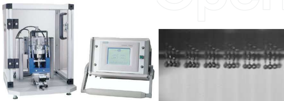
Fig. 2. The Topspot/E (left) and the formation of droplets from the print head (right).
