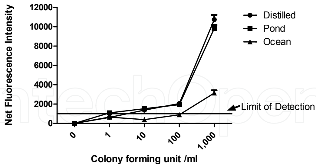
Fig. 1. Capture of C. jejuni on Microfil V filters prior to polymyxin B EIA detection. Various water source samples (500 ml) were spiked with different concentrations of C. jejuni and then filtered. Net fluorescence intensity was obtained by subtraction of background. Means \pm standard error of the means (n= 6 replicates) are plotted as a function of original bacterial concentration.
