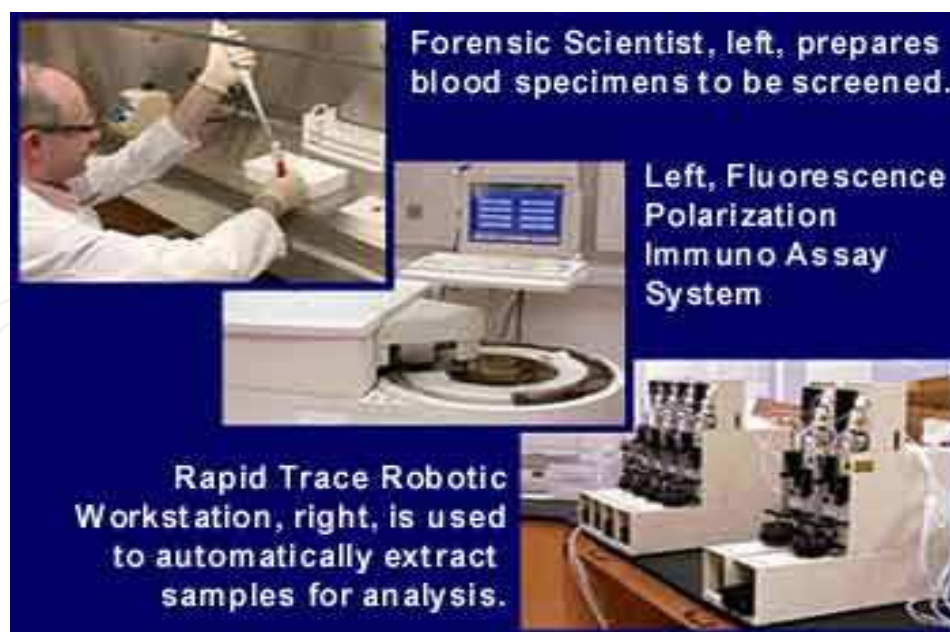
Fig. 4. Rapid trace robotic workstation used in forensic lab.
