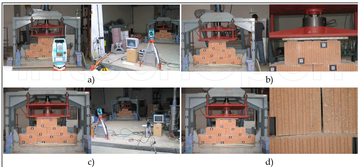
Fig. 10. Test procedure: a) initial coordinates measuring (total station & VMS), b) loading, c) displacement measuring, d) end of test
