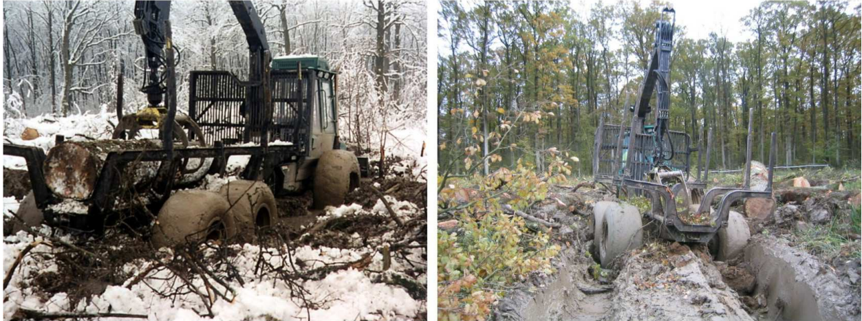
Fig. 1. Forwarder mobility and soil disturbance in main felling of lowland even-aged forests of Croatia
