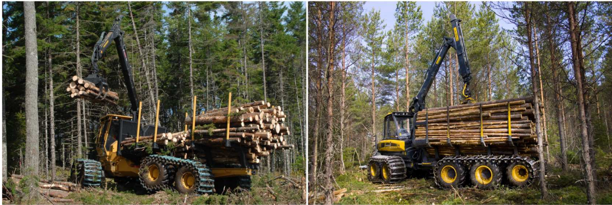
Fig. 8. Eight and ten wheeled forwarder with semi-tracks
