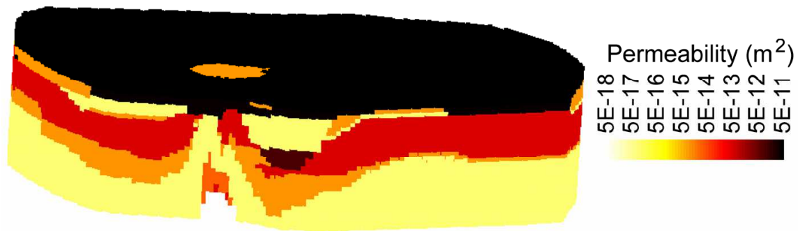
Fig. 5. Gorleben model. Block diagram. Vertical exaggeration ratio 12:1
