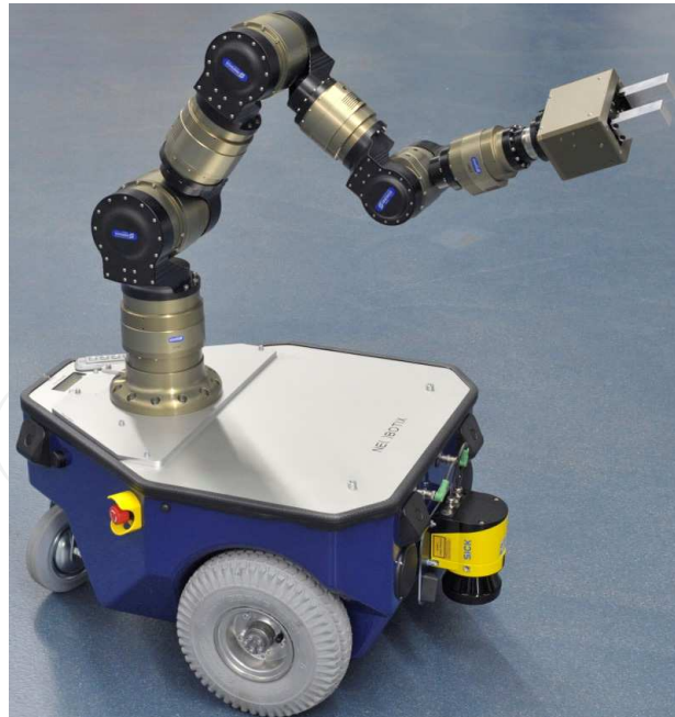
Fig. 14. Assembly of Schunk robotic arm mounted on the Neobotix Platform
