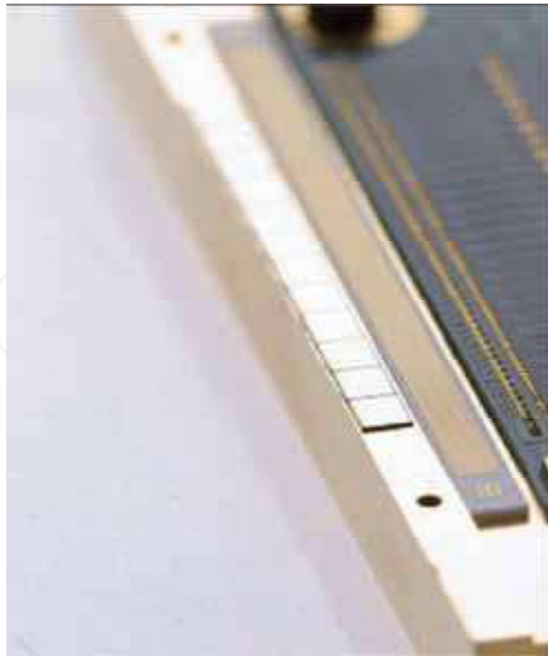
Fig. 17. Photograph of a DLAM 'super-array' comprising a number of monolithic array chips bonded on a common carrier, with the pitch between arrays maintained across the entire print head.
