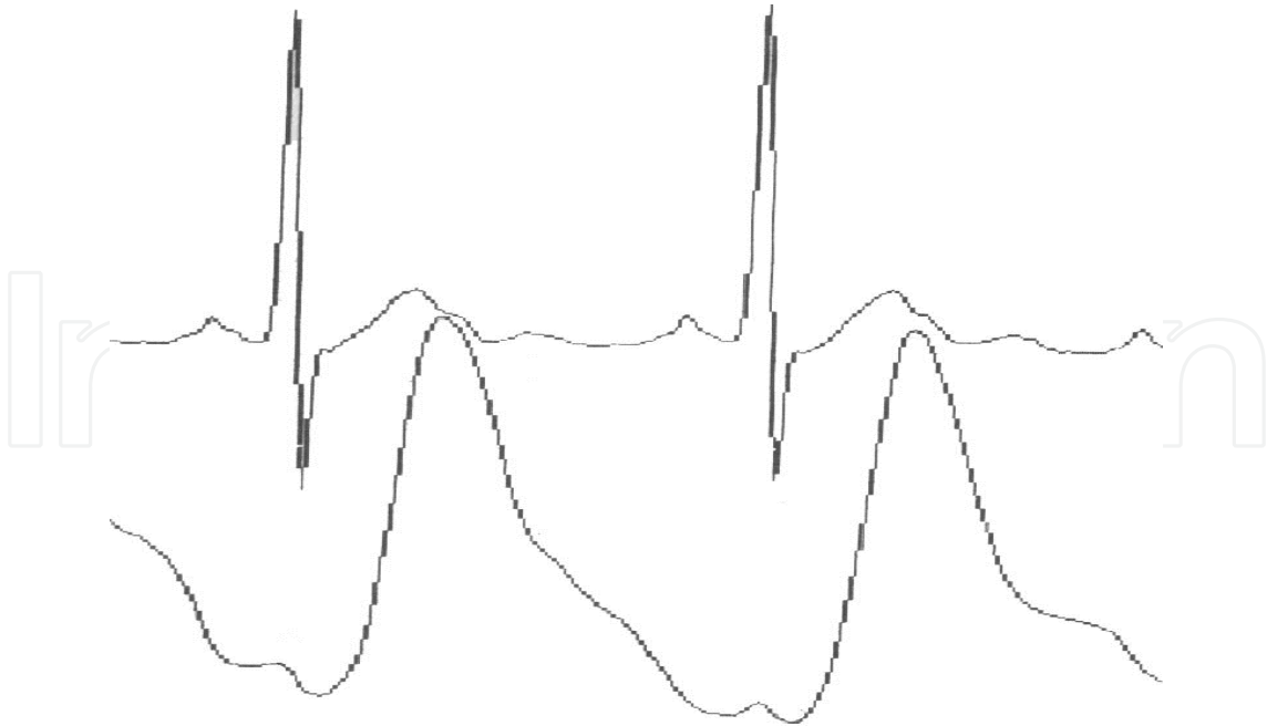
Fig. 3. Arterial pressure wave shape reography-recorded. ECG recorded simultaneously with Rheogram.
