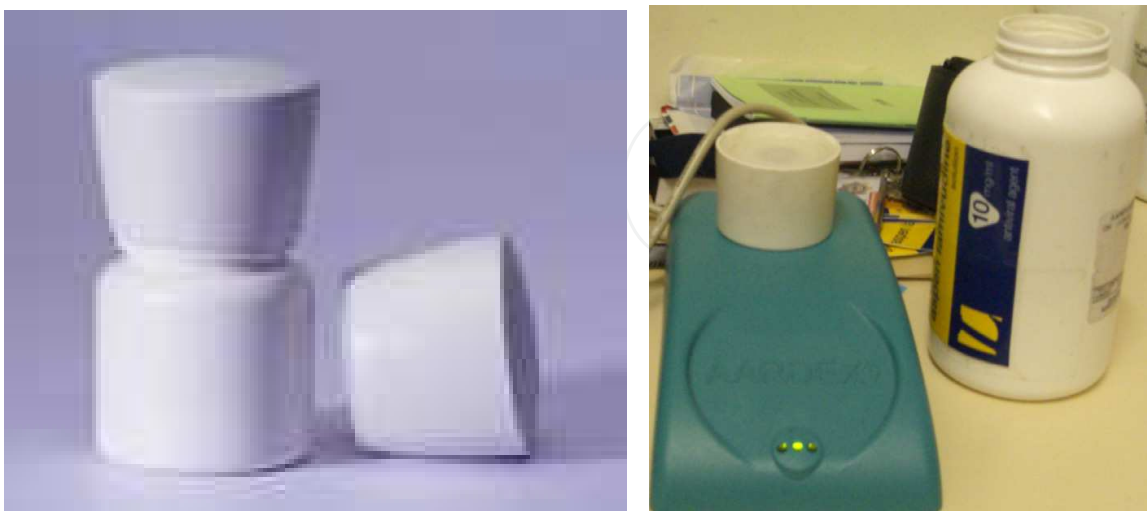
Fig. 2. MEMS container with cap and MEMS terminal to read the microchip
