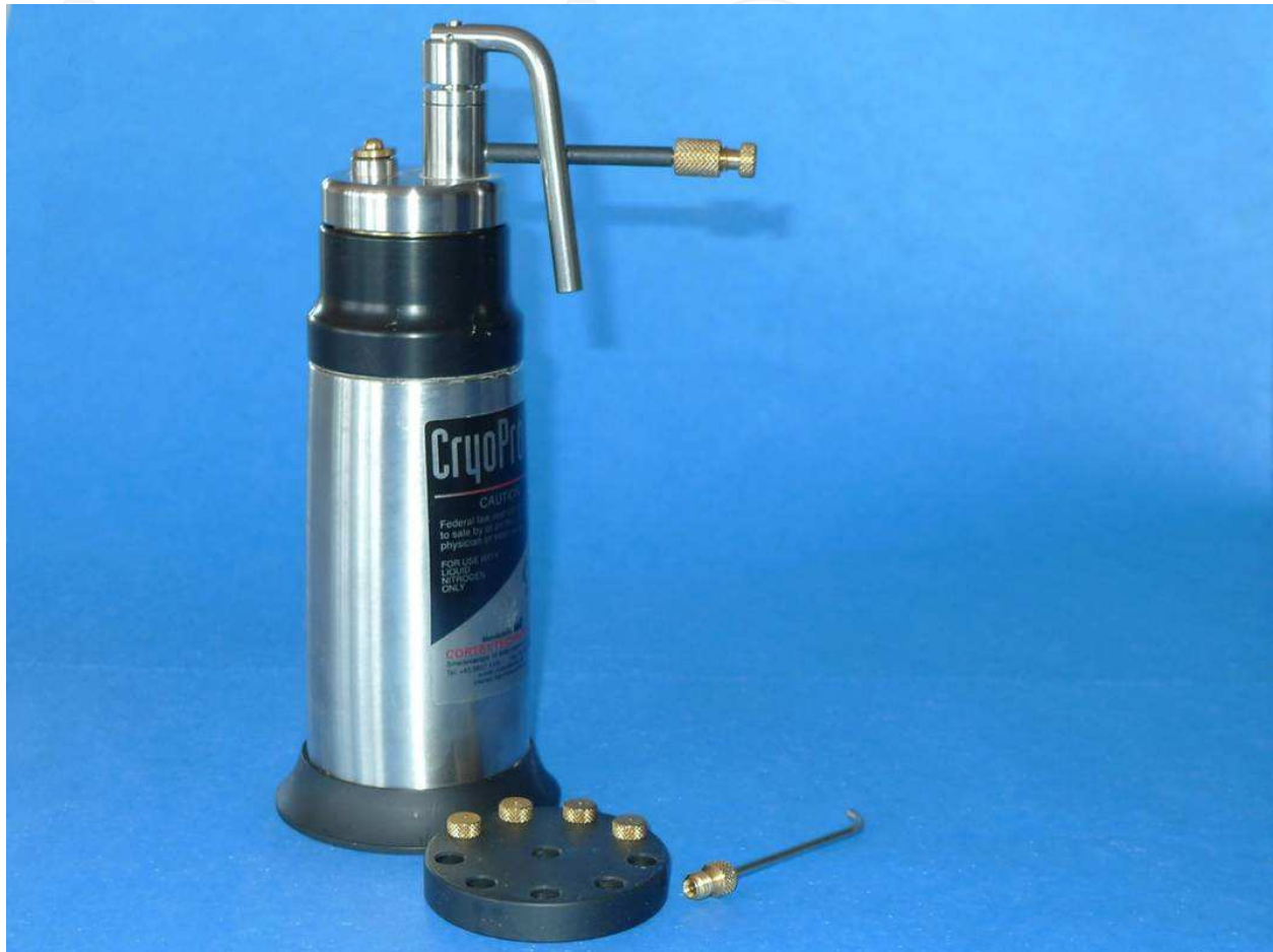
Fig. 5. Equipo de criocirugía. Portable unit of cryosurgery for liquid nitrogen. It consists of a thermos of stainless steel, covered with a structure of bronze and stainless steel, with a special system of valves and a great mouth of filling, the pulverization being controlled by means of a trigger. They are light and of easy transport.
