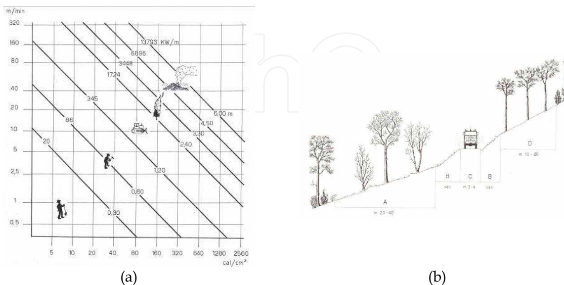
Fig. 3. Fire Behaviour Characteristics Chart (a) and one example of preventive action (b)
