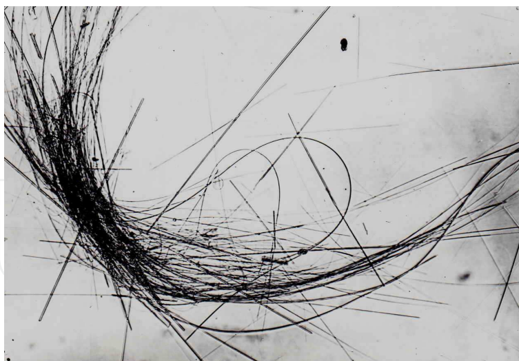
Fig. 10. Micrograph of synthetic fibrous fluorosilicates (x 110).
