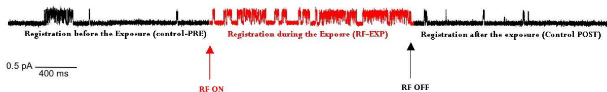
Fig. 2. Single channel current recorded before, during, and after the exposure to RF field
