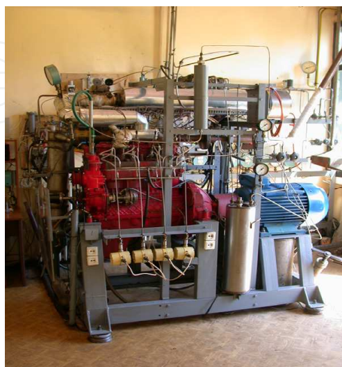
Fig. 8. Д-245 diesel-based synthesis gas generator.
