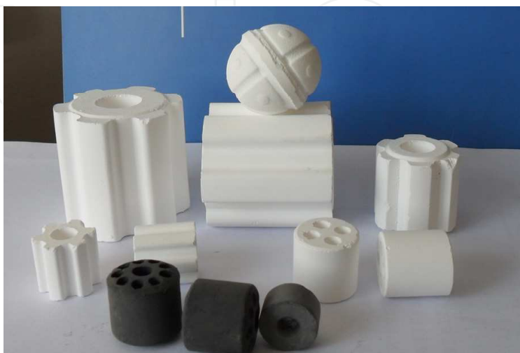
Fig. 5. The novel shapes with high strength of the reforming catalyst and support.
