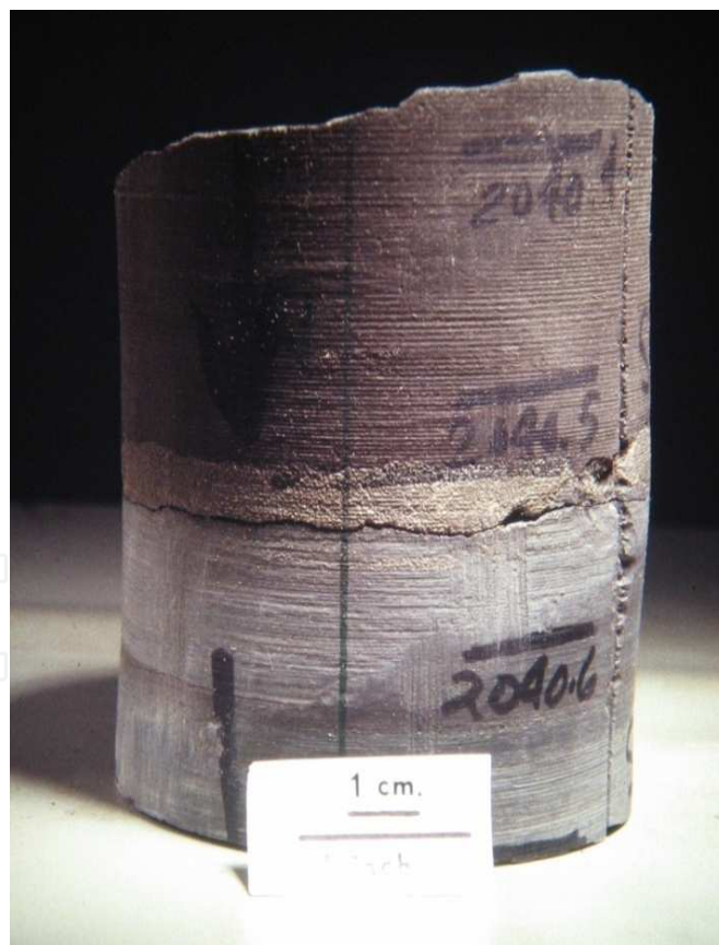
Fig. 4. Black Cleveland Shale above gray Chagrin Shale in an EGSP core from Ohio, with pyrite at the contact (2040.54 ft.). An orientation groove is visible to the right of the depth marks; the vertical line on the front of the core marks north. Photo by Daniel J. Soeder.
