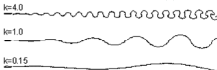
Fig. 4. Computed vortex traces as a function of the reduced frequency k , \alpha = 2.5 + 4\sin(\omega t)
