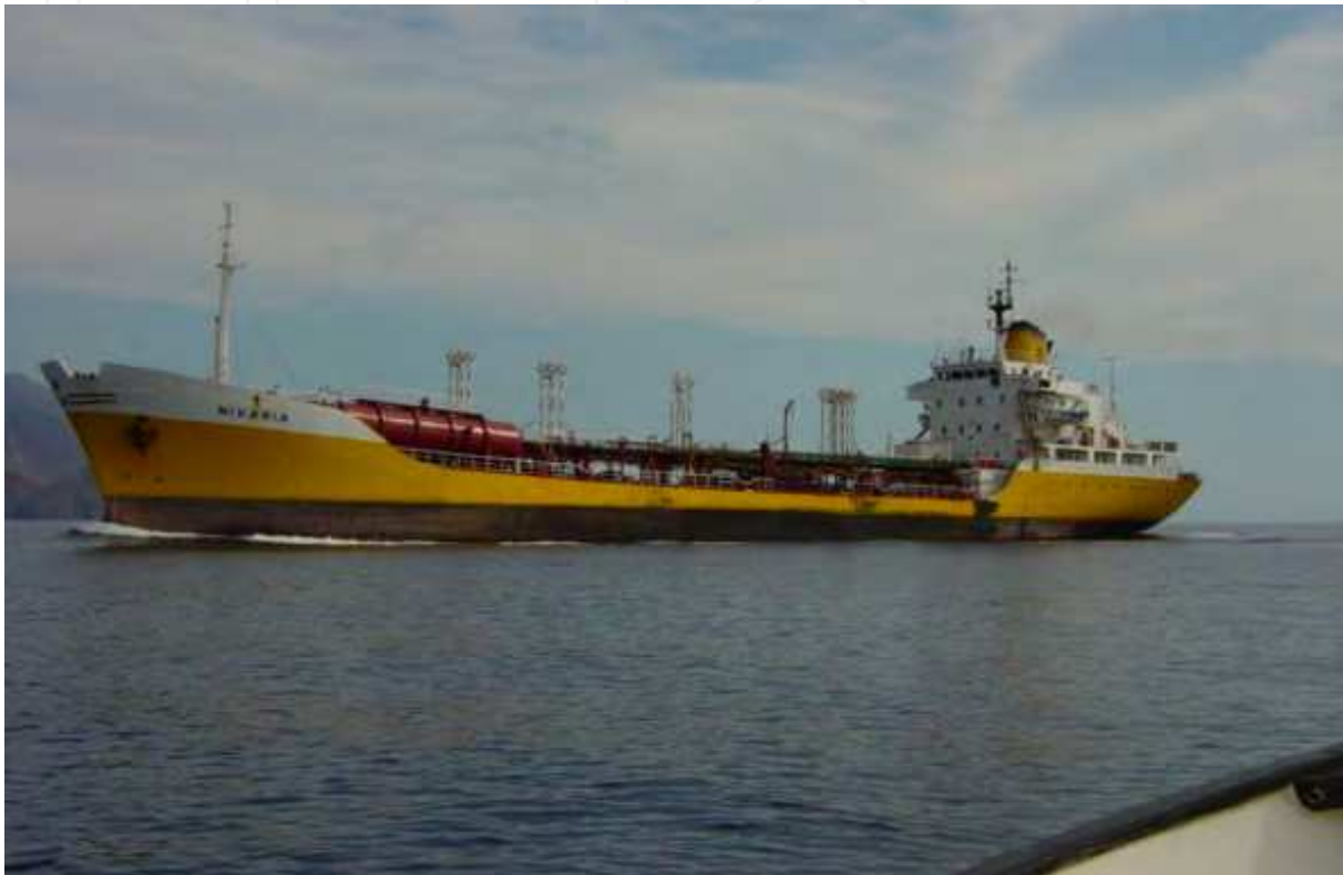
Photo 4. Carrier need ballast (water) when they travel without cargo in order to keep their stability
