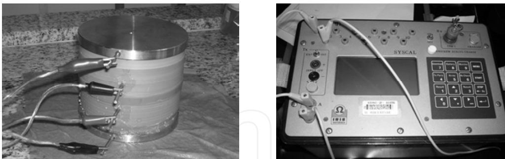
Fig. 16. Instrumented undisturbed specimen and Syscal Pro equipment used for laboratory electrical resistivity measurements (Mondelli et al., 2010a).
