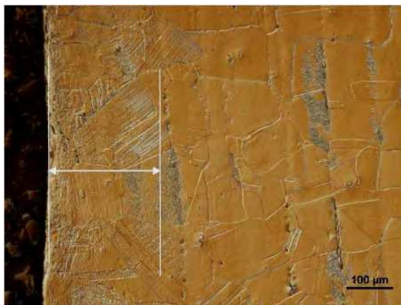
Fig. 12. Plastic deformation of the surface to a depth of 220 \mu\text{m} , local plastic deformation in the austenitic grain, zone of hole H
