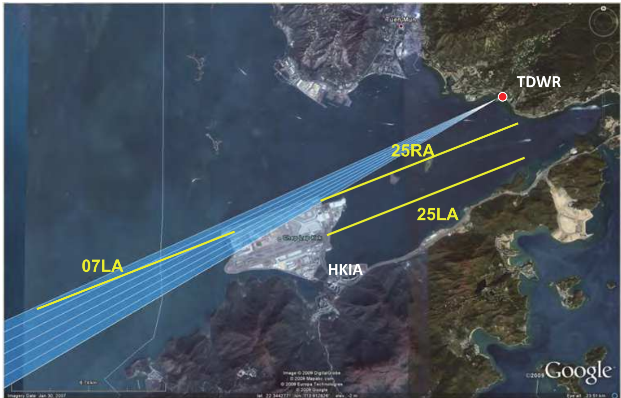
Fig. 1. The locations of the Hong Kong TDWR (red dot) radar and Hong Kong International Airport (HKIA). The blue beams illustrate the radar beams over the runways corridor 07LA of the airport with 1^\circ azimuth interval. Three yellow lines indicate the approach paths and their names are marked.
