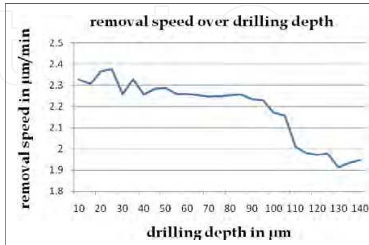
Fig. 20. Removal speed over drilling depth
