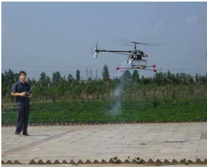
Fig. 9. ServoHeli-20 fault detection experiment
