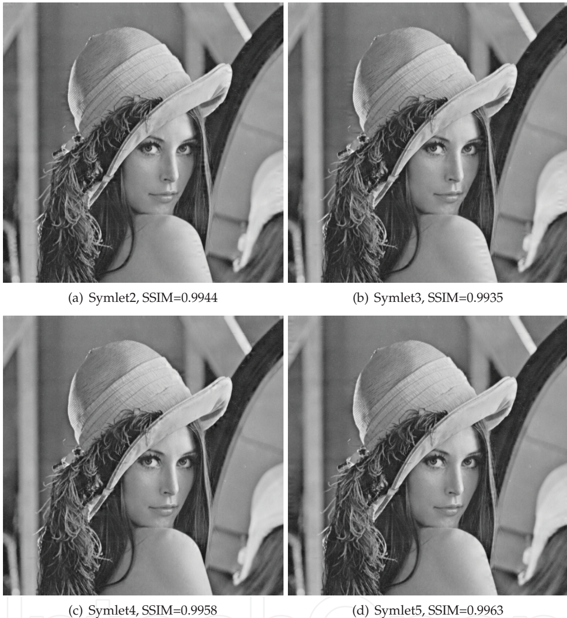
Fig. 8. Test image Lena watermarked using different gradient transforms in the GDWM method. In each case, a 256-bit watermark is embedded with PSNR=42dB.
