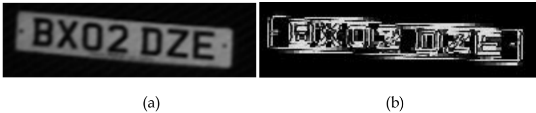
Fig. 9. The original license plate candidate image is shown in (a) and prominent edges in the LP candidate are shown in (b) two levels decomposition
