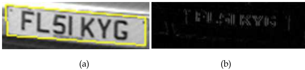
Fig. 12. (a) The input LP Candidate f(x,y) and (b) the detected edges using 2D Haar WT E(x,y)
