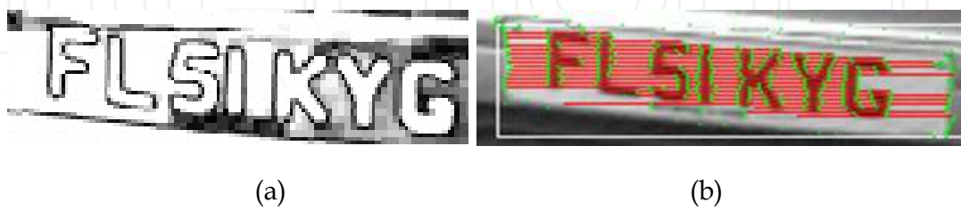
Fig. 13. (a) The post- processed 2D Haar WT edges E_{Haar} and (b) the detected edges in green E_{FIN}
