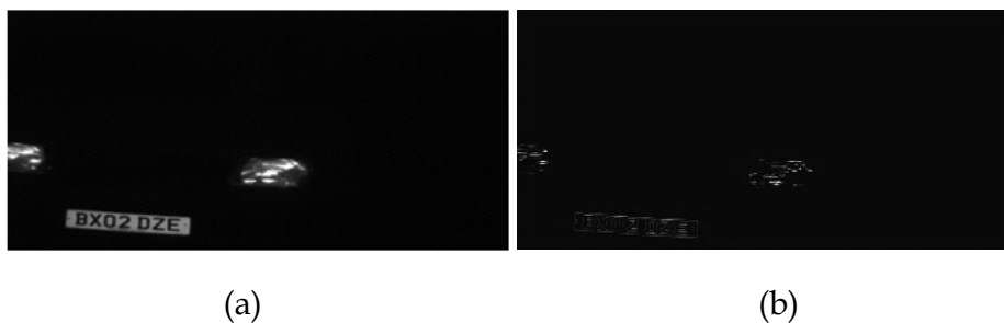
Fig. 6. The original image is shown in (a) and the resulting image from reconstruction using single level IDWT is shown in (b)
