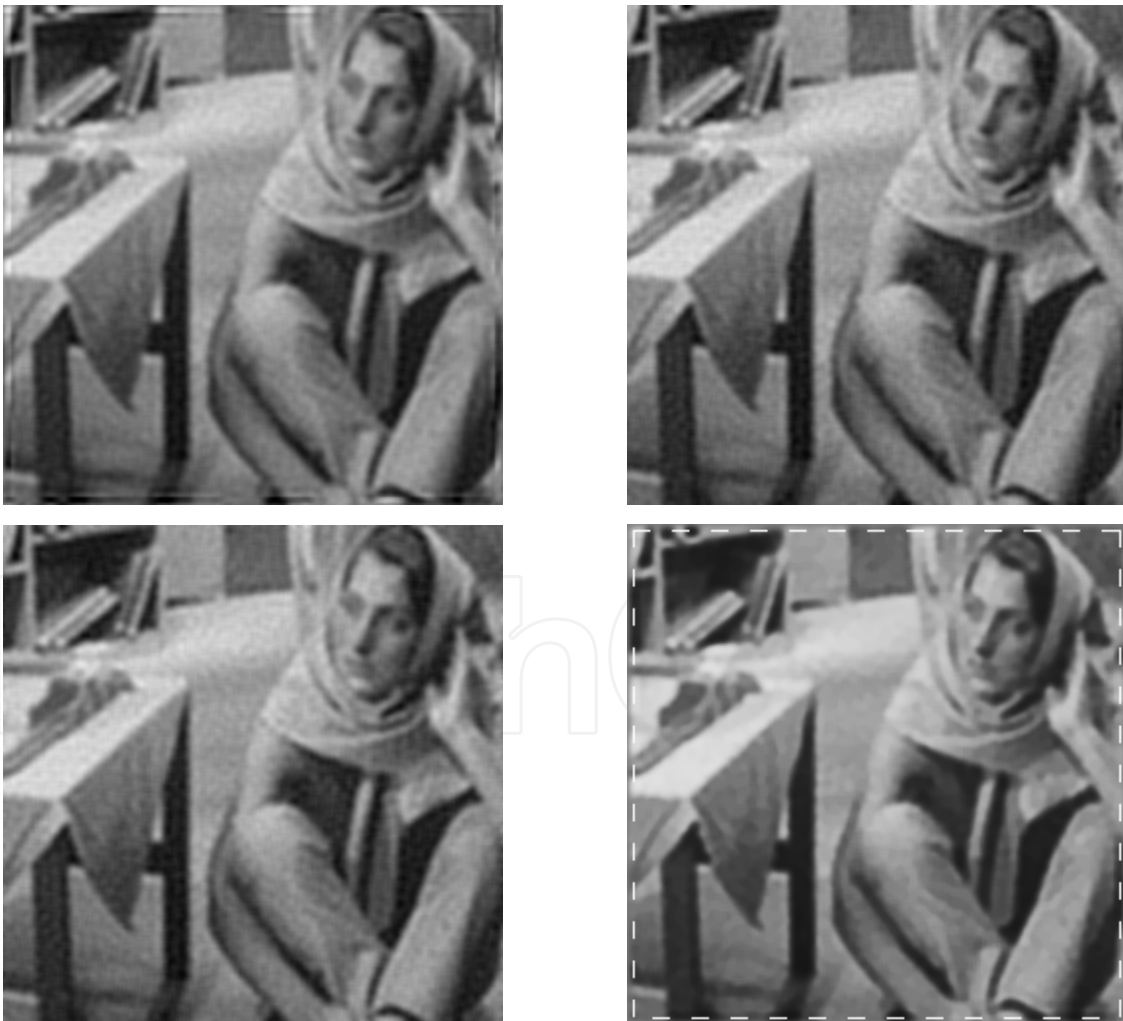
Fig. 8. Restored images with HyBR under periodic (upper-left), reflective (upper-right) and anti-reflective (bottom-left) BCs. Restored image with our MLP (bottom-right).
