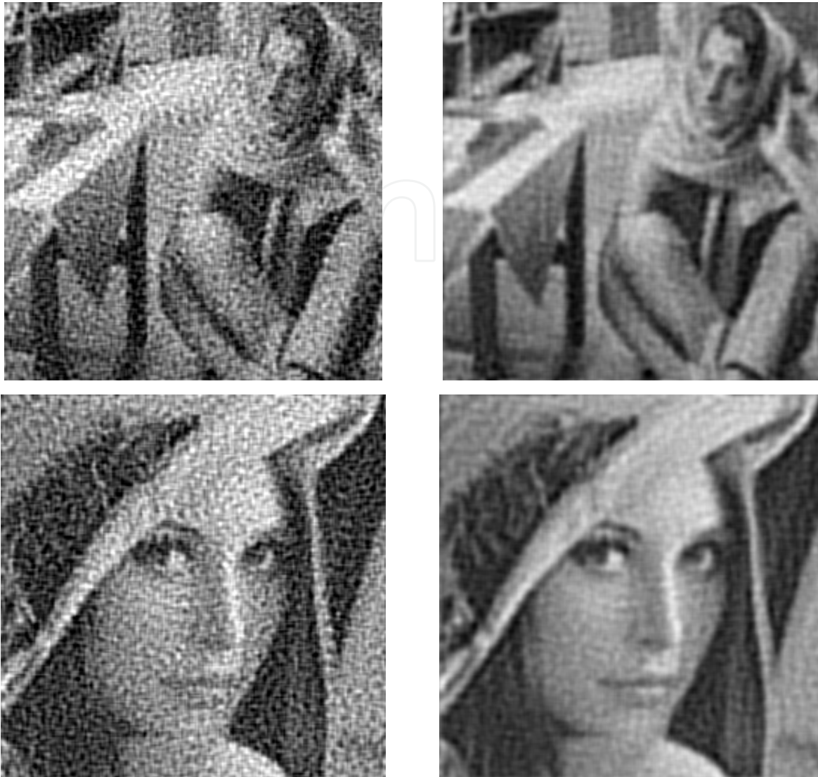
Fig. 12. Restored images with Tikhonov filter (upper-left and bottom-left) compared to the restored images of the desensitization filter (upper-right and bottom-right).
