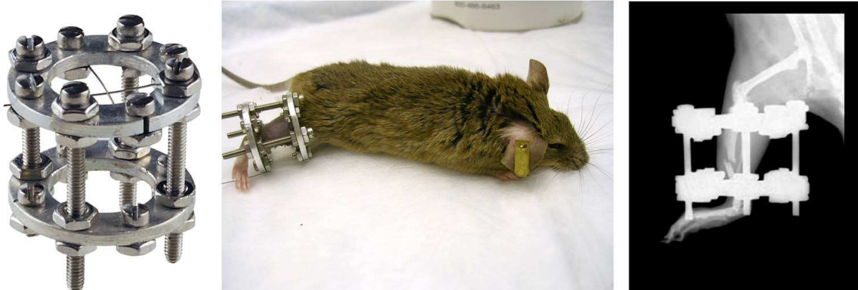
Fig. 10. Mini Ilizarov circular frame applied to a mouse model of DO in our laboratory , and developed by Tay et al. (Tay et al., 1998).
