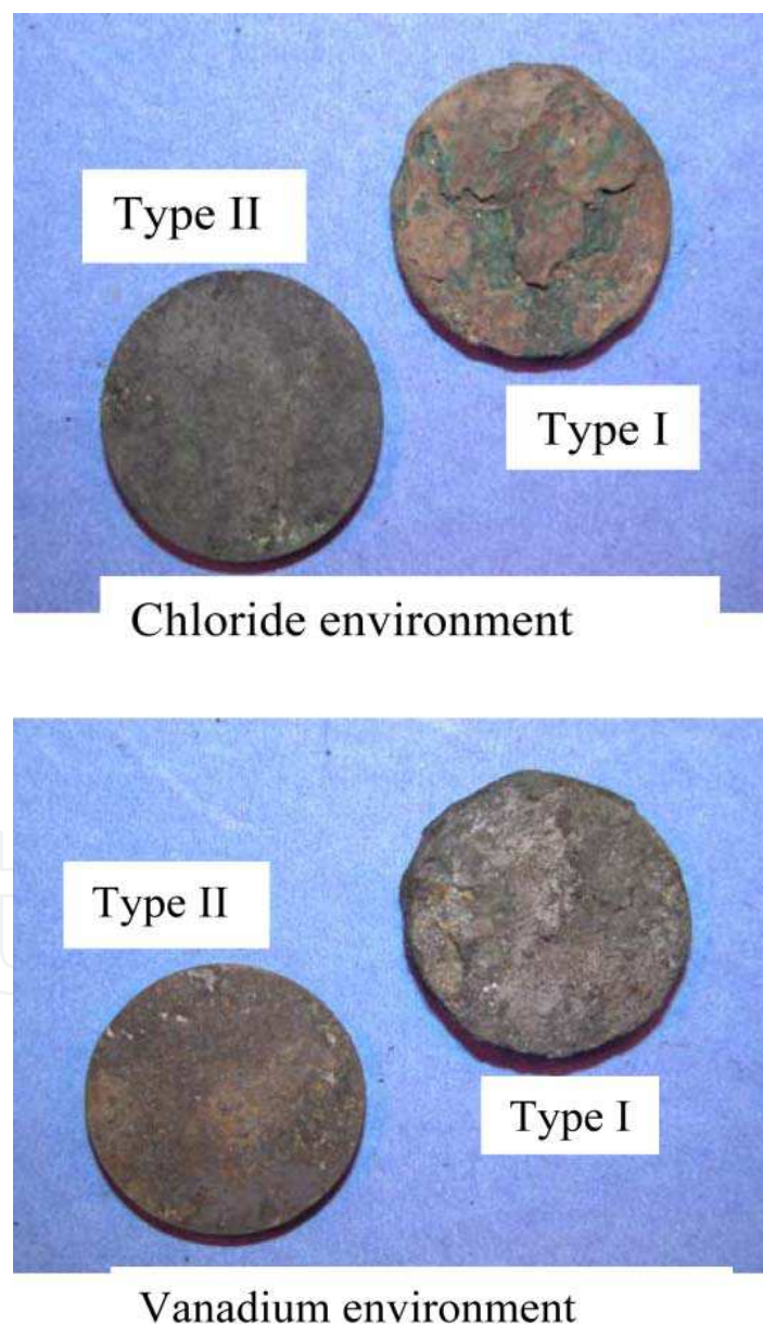
Fig. 3. As hot corroded superalloy SU-263 in marine and vanadium containing environments under type I and type II conditions
