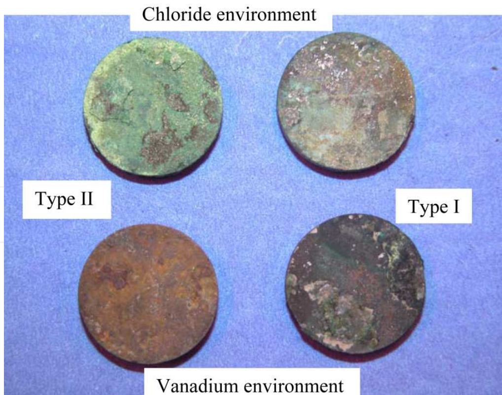
Fig. 5. As hot corroded superalloy IN 738 LC in marine and vanadium containing environments under type I and type II conditions
