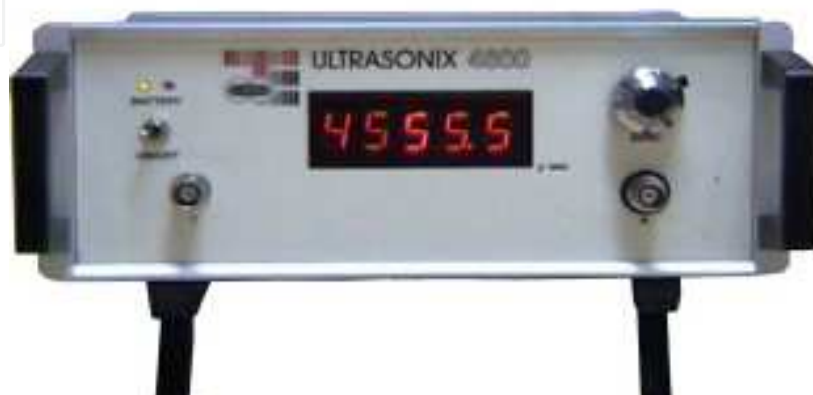
Fig. 6. Compressional wave velocity (P-wave) measuring device 'Ultrasonix 4600'
