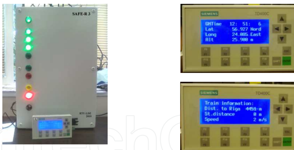
Fig. 20. Functional prototype and information screen with satellite navigation data
