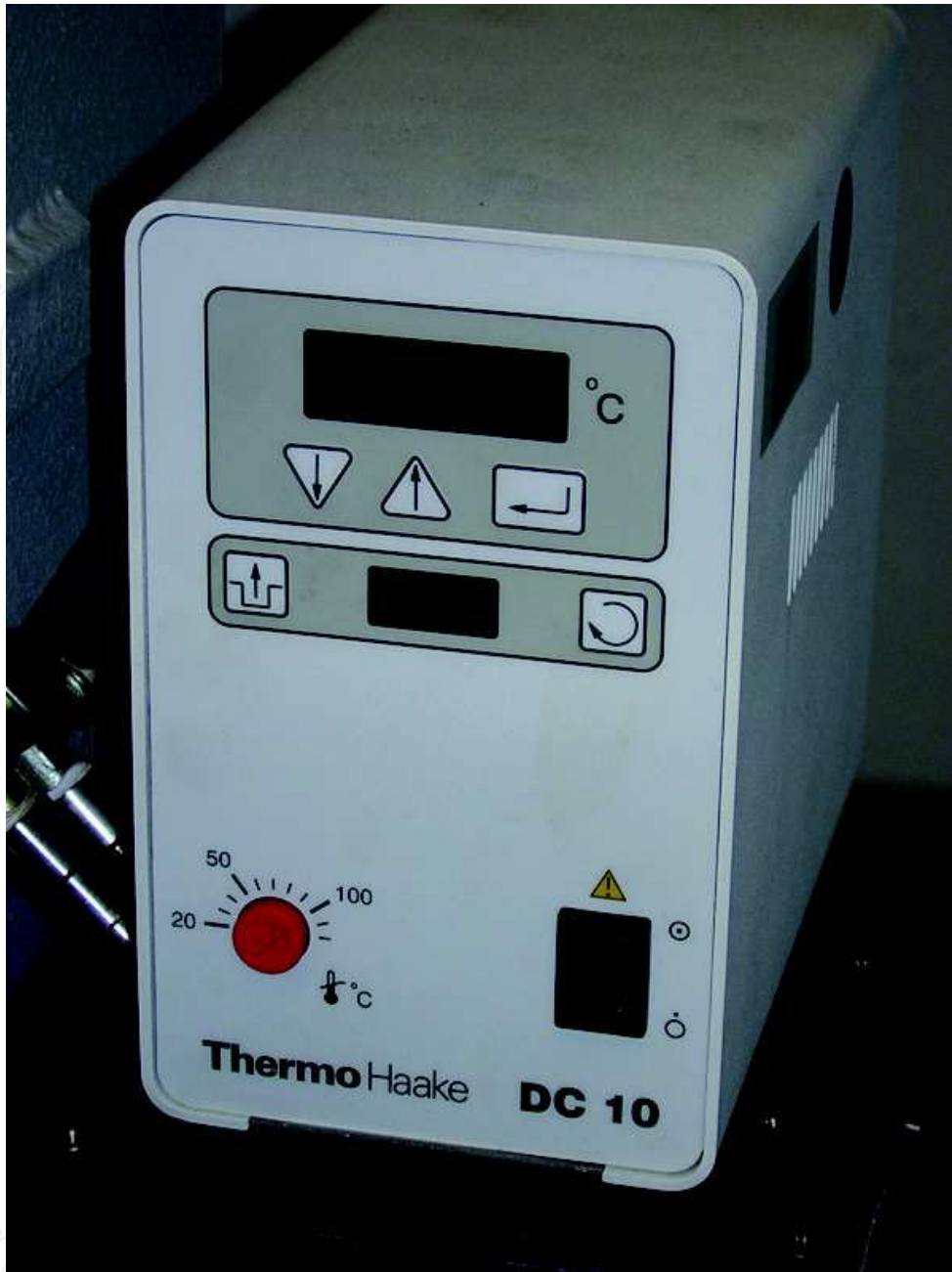
Fig. 4. Temperature control unit (Thermo Fisher Scientific, Karlsruhe, Germany). Open bath circulator with digital settings, bath vessel and bath bridge made of stainless steel and temperature resistant polymer; electronic control using a digital sensor for predetermined reference value, max. temperature 100 °C.
