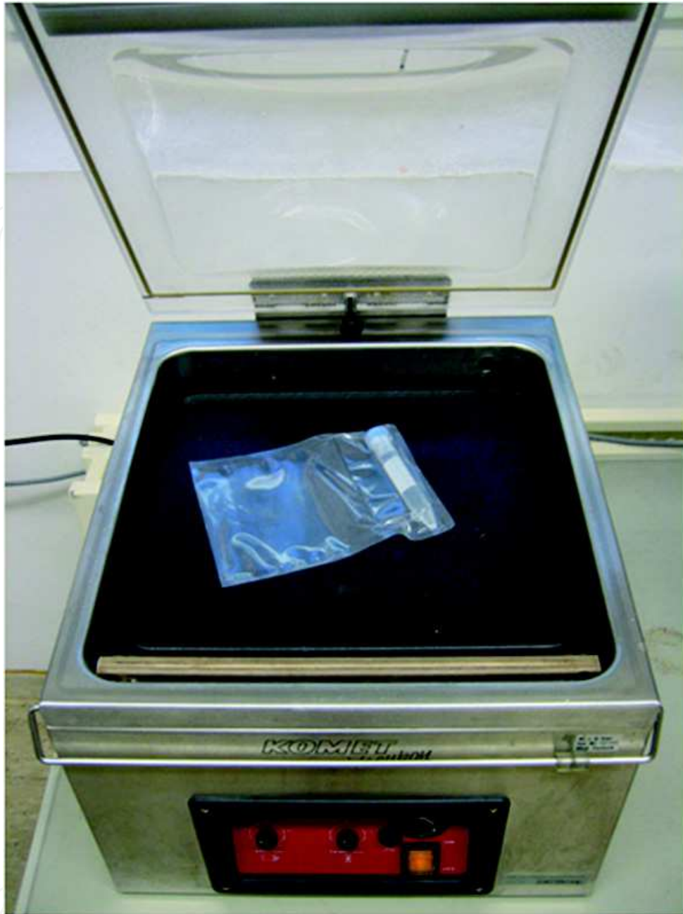
Fig. 2. Vacuum sealing device (Komet, Plochingen, Germany). Specimens in polyethylene bags are placed into the vacuum chamber, positioning the open section onto the sealing bar. Once a vacuum is formed a heated wire on the bar seals the plastic bag. On the control board vacuum and sealing settings can be adjusted individually.
