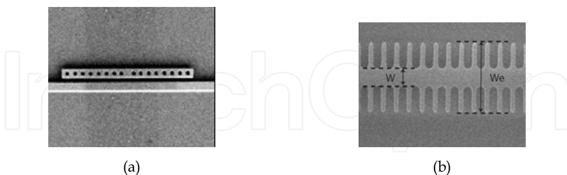
Fig. 2. SEM pictures of two planar 1D periodic structures used for sensing purposes. (a) 1D SOI holes cavity (Goddard et al., 2010); (b) 1D SOI corrugated waveguide (Castelló et al., 2011).
