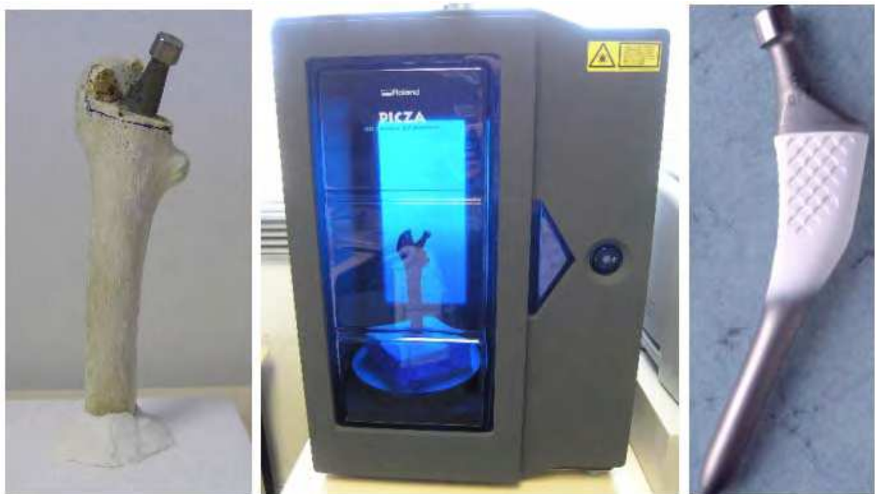
Fig. 1. Real model of an implanted femur, 3D laser scanner and femoral stem
