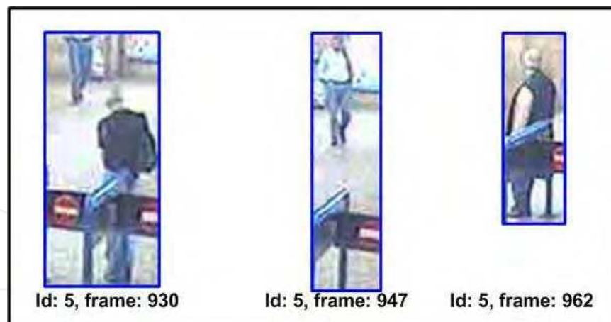
Fig. 8. An example of object ID confusion: three ground-truth object IDs associated to one sole detected object (object ID confusion = 3).
