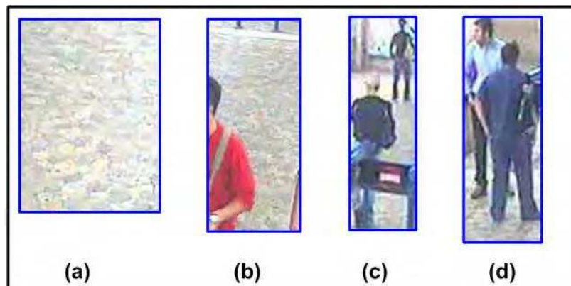
Fig. 6. Examples of object detection quality (a) The object is not present in the blob; (b) The object is partially present in the blob; (c) and (d) The object is totally present in the blob.
