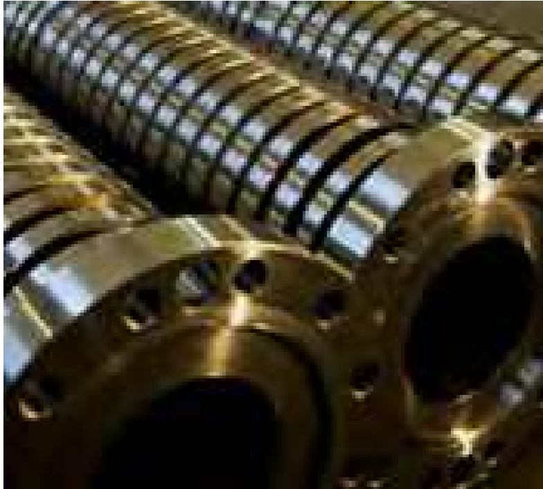
Fig. 25. Extruder screw, Cronidur 30 [ETE-11].
