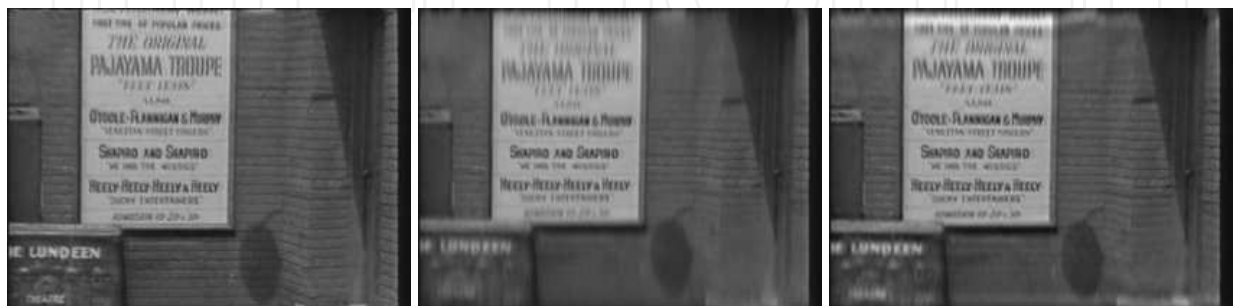
(a) The original input - 280 \times 210 pixels. (b) The result of applying the Green's matrix over the original input. (c) The result of motion reversal.
