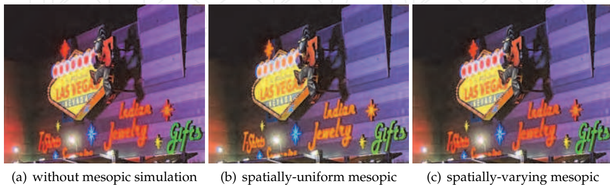
Fig. 16. Comparison between an image without mesopic simulation (a), with global mesopic filter (b) and per-pixel mesopic filter (c). All red intensities shift toward orange/yellow in (b), while only those not sufficiently bright enough change in (c) like the light reflex in the leftmost wall. Also note that purple tones shifted towards a more blueish hue in the mesopic images.
