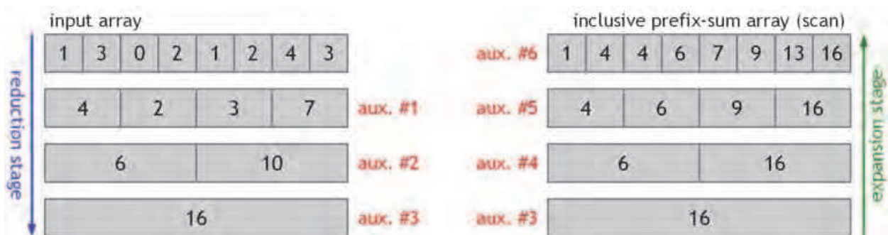
Fig. 11. Suggested layout for the auxiliary GPU memory during the scan. Simultaneous read/write from/to a same buffer never happens. In order to expand aux.#4 the expanded parent buffer aux.#3 and the reduced sibling buffer aux.#2 must be accessed. Similarly, expanding aux.#5 needs access to aux.#4 and aux.#1. The final expansion uses aux.#5 and the input buffer itself. The extra memory amounts to about three times the size of the input.
