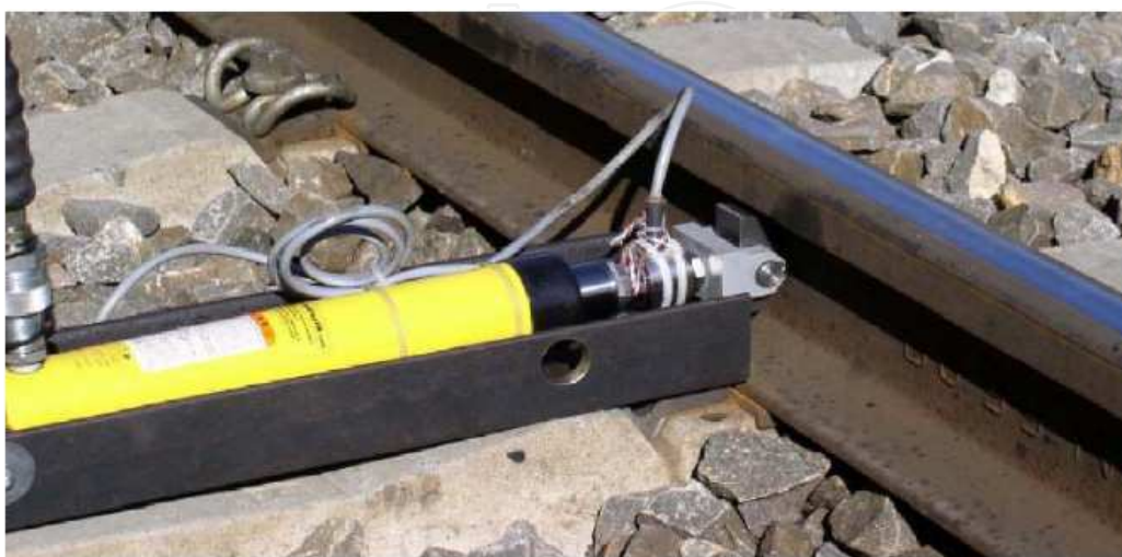
Fig. 12. The Device that applied the lateral force to the track
