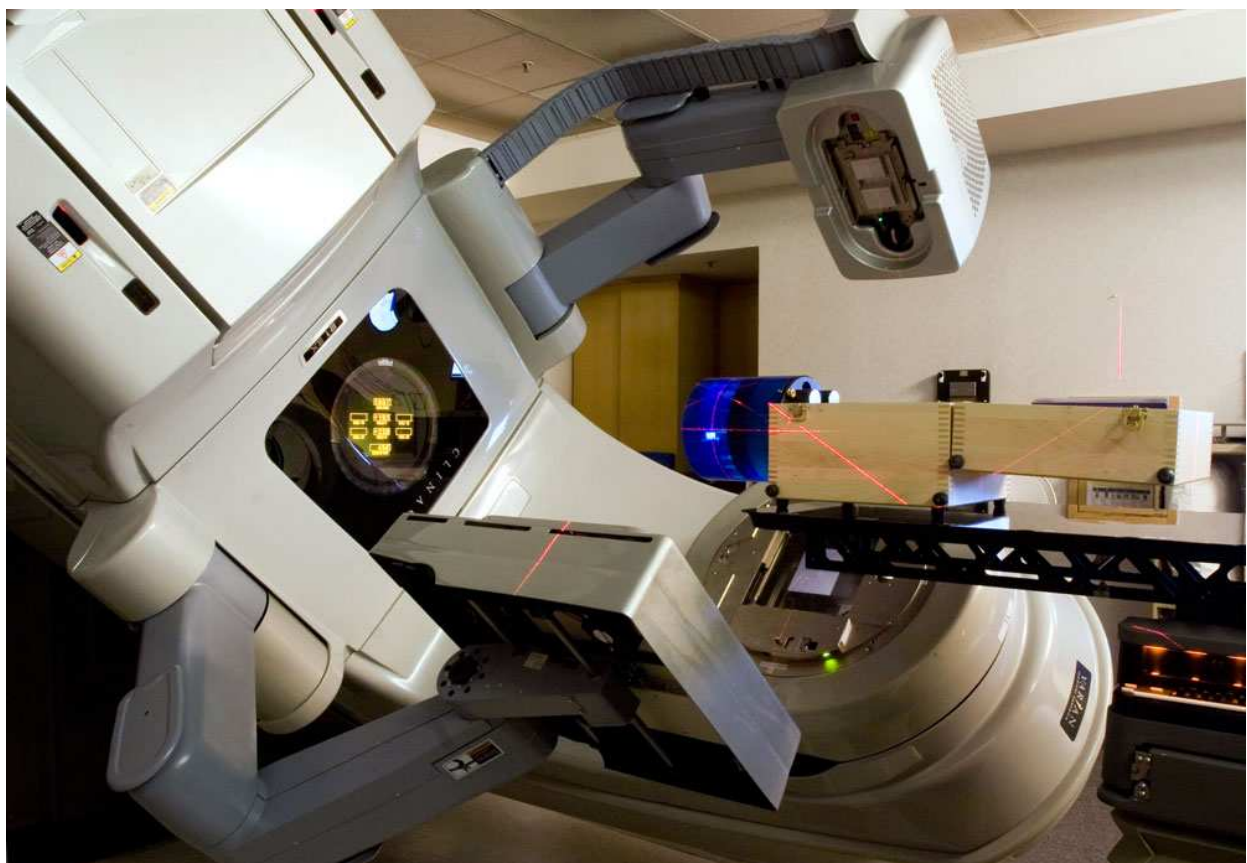
Fig. 10. Setup of Catphan at machine Isocenter to be imaged for image quality tests.
