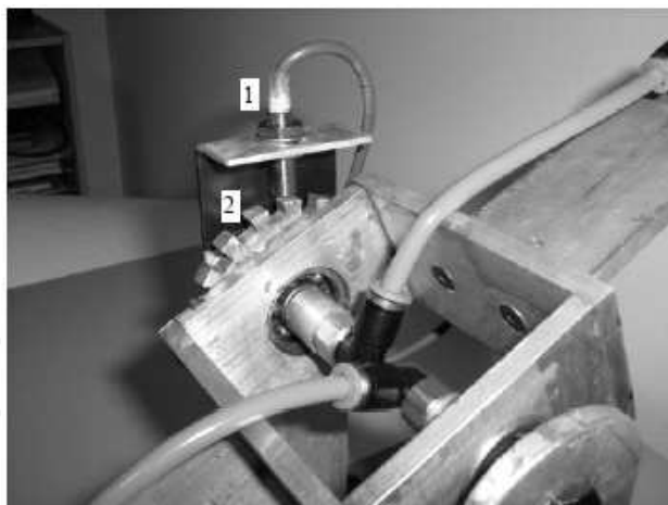
Fig. 19. Close-up view of the inductive proximity sensor and gear assembly. i) Inductive proximity sensor and ii) 18 teeth gear
