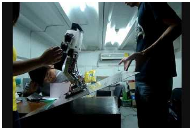
Fig. 13. Robot Inclined Steel Plate Balancing Experiment. Front position. Note that the hand of the person is not touching the robot. This is just in preparation to catch the robot when it falls.
