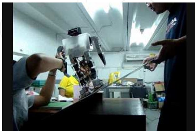
Fig. 11. Robot Inclined Steel Plate Balancing Experiment. Left position. Note that the hand of the person is not touching the robot. This is just in preparation to catch the robot when it falls.
