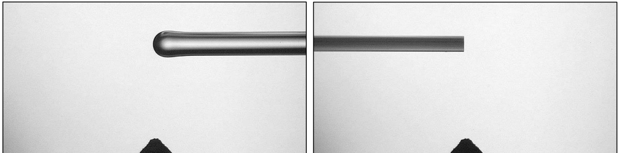
Fig. 27. Left: SMF tip melted - Phase 2. Right: PCF positioned for melting.
