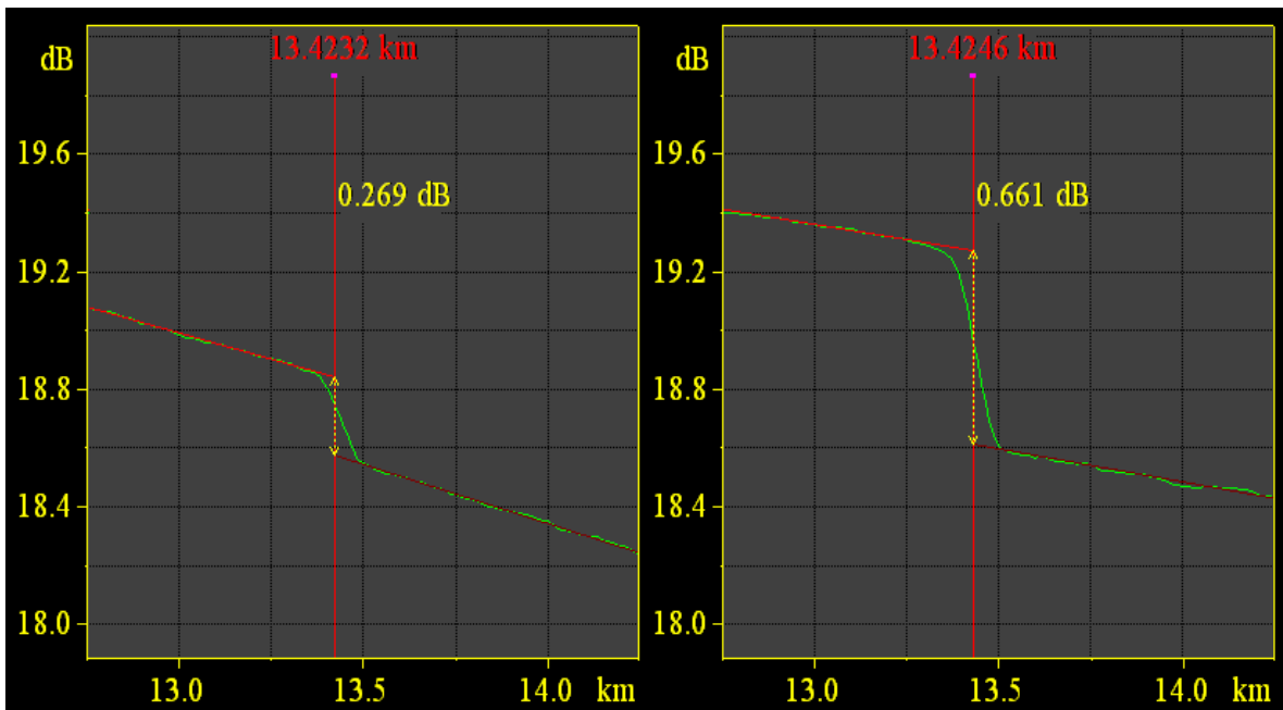
Fig. 8. Sharp bend of SMF observed with OTDR at 1310 nm (left) and 1550 nm (right).
