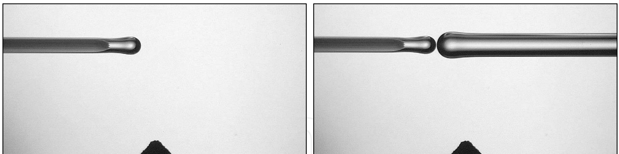
Fig. 28. Left: PCF tip melted. Right: fibres aligned for fusion with axial offset.
