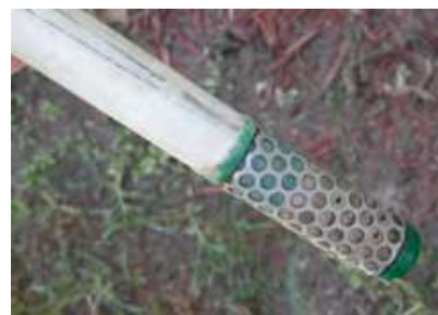
soil moisture sensor glued to PVC pipe
