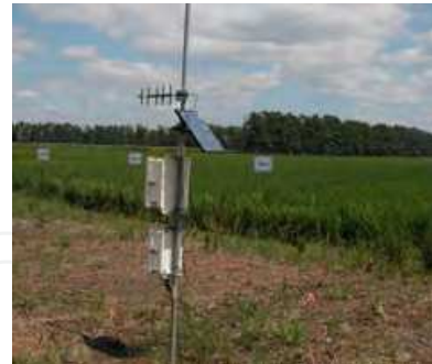
datalogger and transmitter
