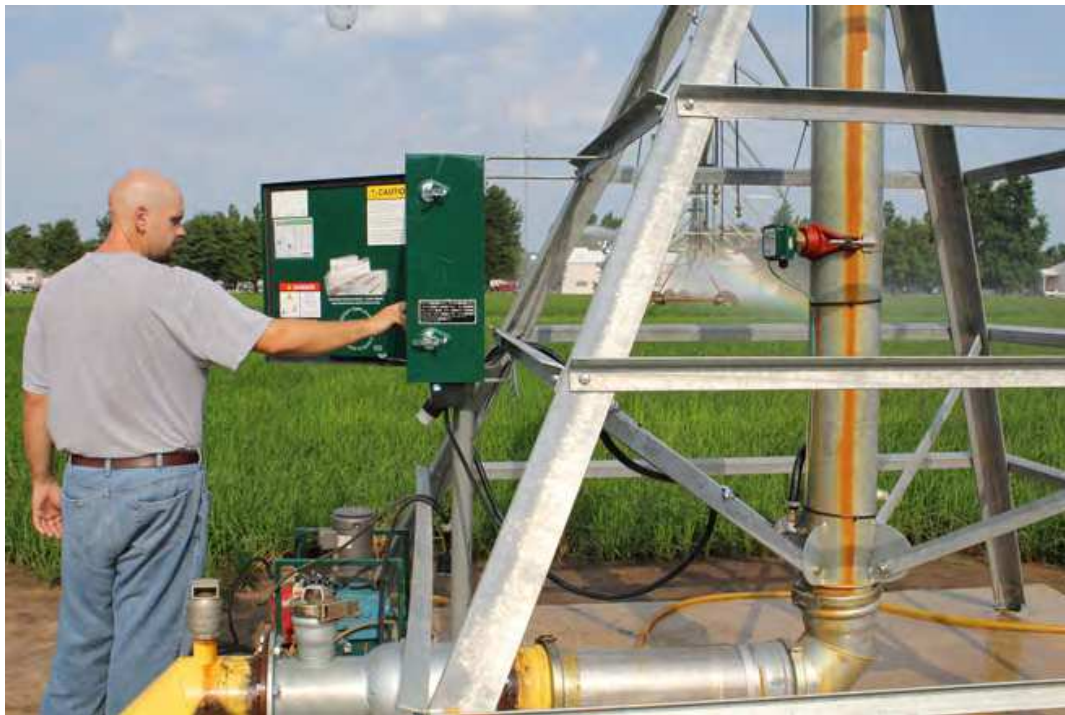
Fig. 1. Center pivot irrigation system equipped with a backflow prevention valve used to apply irrigation water, and an injection pump for applying liquid nitrogen fertilizer and fungicides for controlling diseases.
