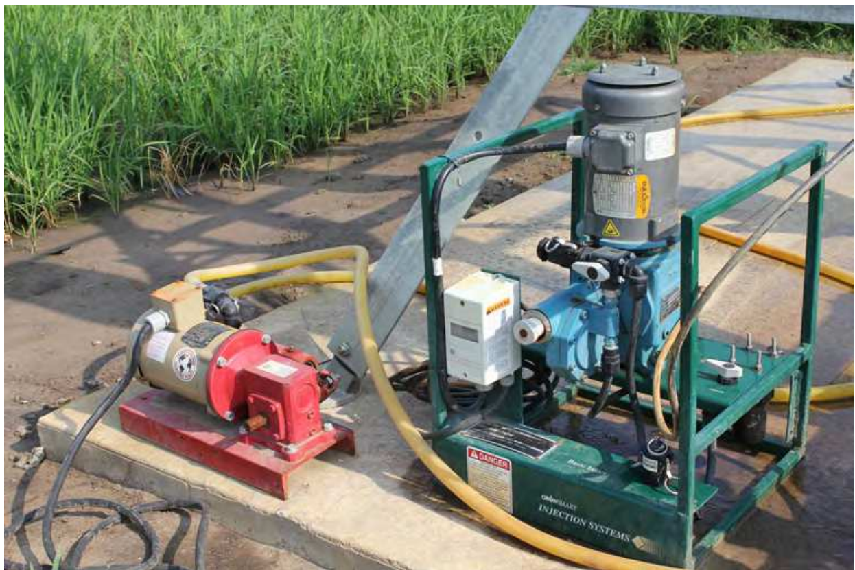
Fig. 12. Two types of injection pumps commonly used for chemigation. The pump on the left is a piston type and the pump on the right is a diaphragm type.
