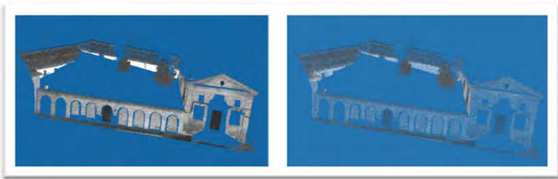
Fig. 7. General scan of the façade before and after applying a 100mm spatial sampling.
