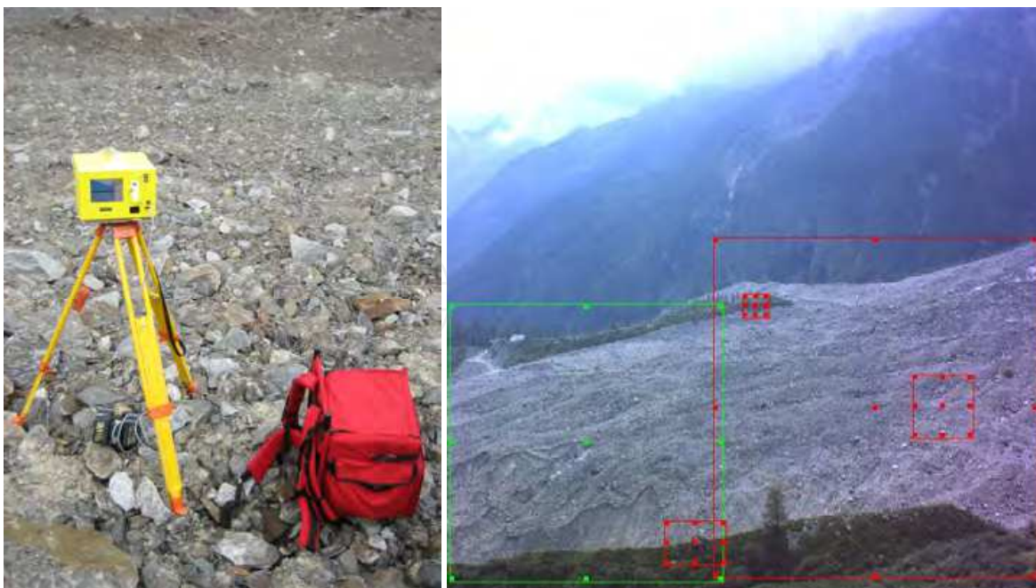
Fig. 5. ILRIS-3D mounted on tripod and the special backpack employed in instrument transport (left) and ILRIS-3D interface control - red squares represent surveyed areas, the green one is the area under measurement (right)
