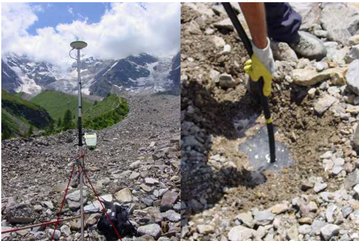
Fig. 11. Installation of an ablation stake using a stream driller and D-GPS measurement (Photo P. Federici)
