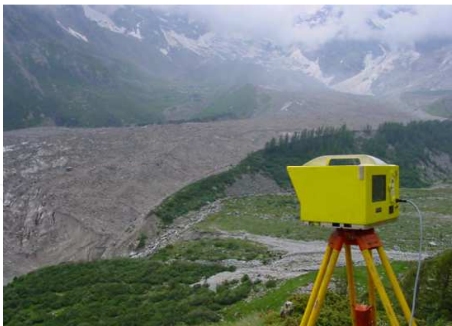
Fig. 4. The Optech ILRIS-3D laser scanner during a field measurements (photo P. Federici)
