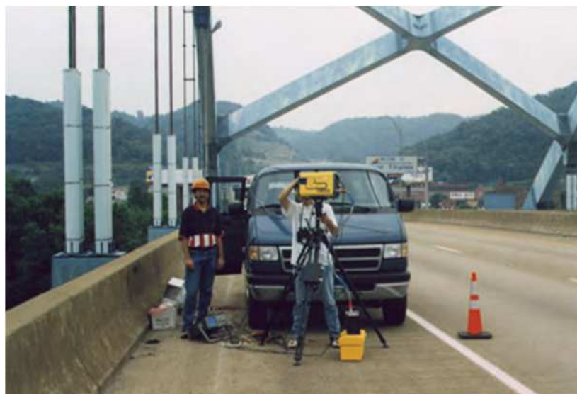
Fig. 14. Cable Vibration Measurements from the Bridge Deck [41] (Chen et al. 2005)
