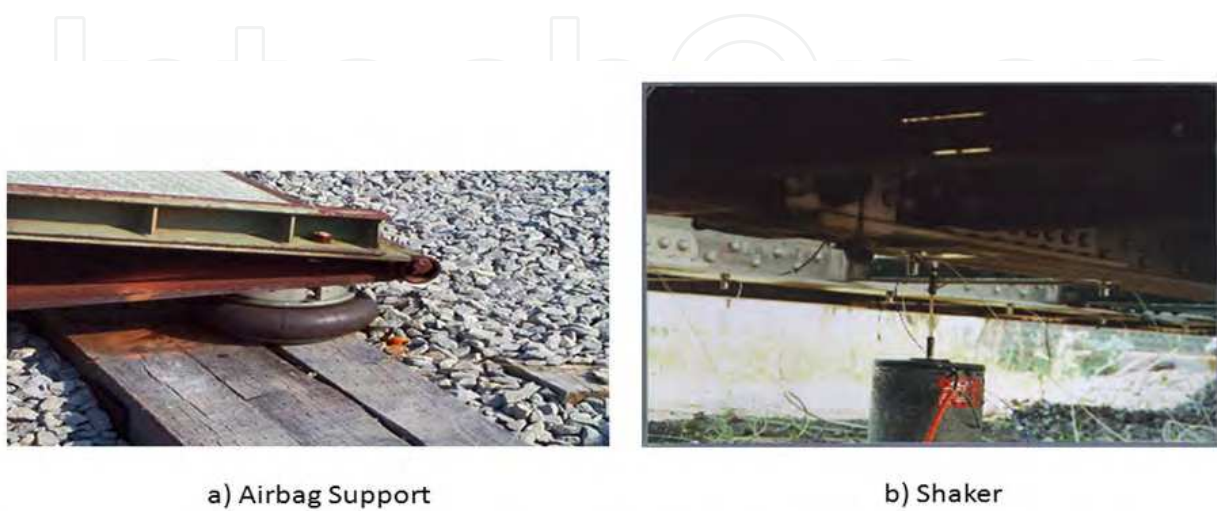
Fig. 12. Testing Setup: a) Airbag and b) Shaker
