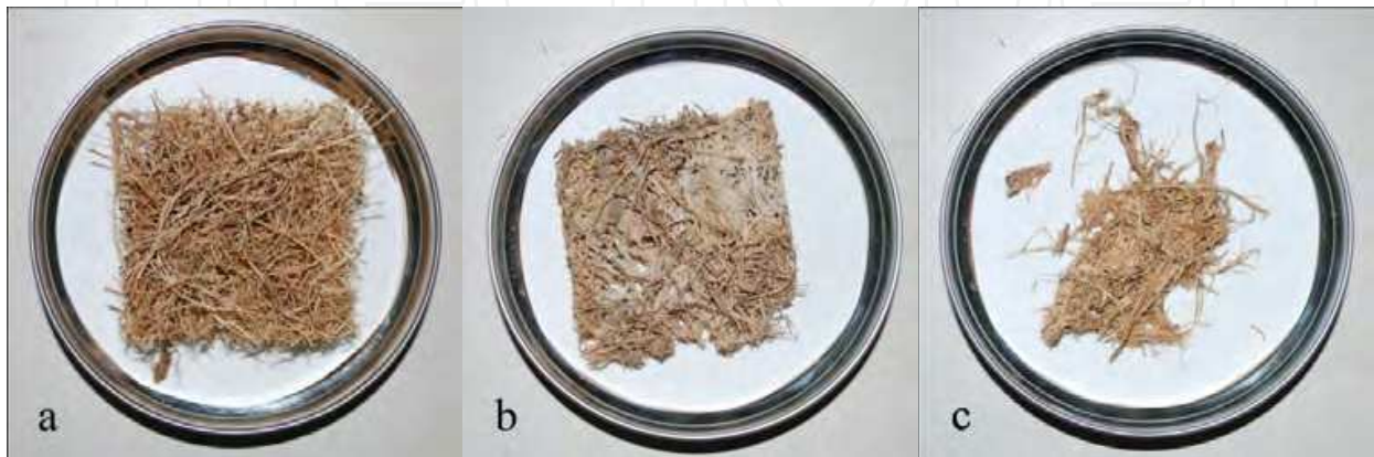
Fig. 16. a) before decay b) decayed ABS coated c) decayed uncoated fibre sheet in the silty sand soil after 3 months
