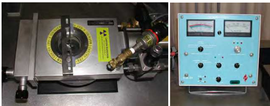
Fig. 2.4. Left: Lumiscope sample holder. Right: Lumiscope control and electronics.
