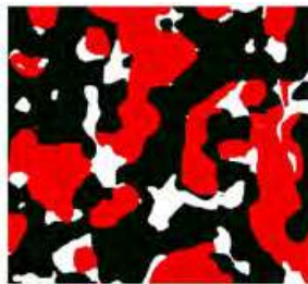
Fig. 2. Two-dimensional FE model of a single cross-section of the SOFC anode
